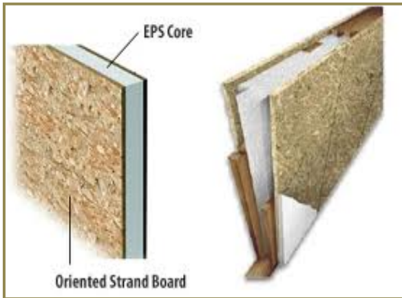
Figure 9: Structural Insulated Panel Detail. Source: www.universalconstructionfoam.com
