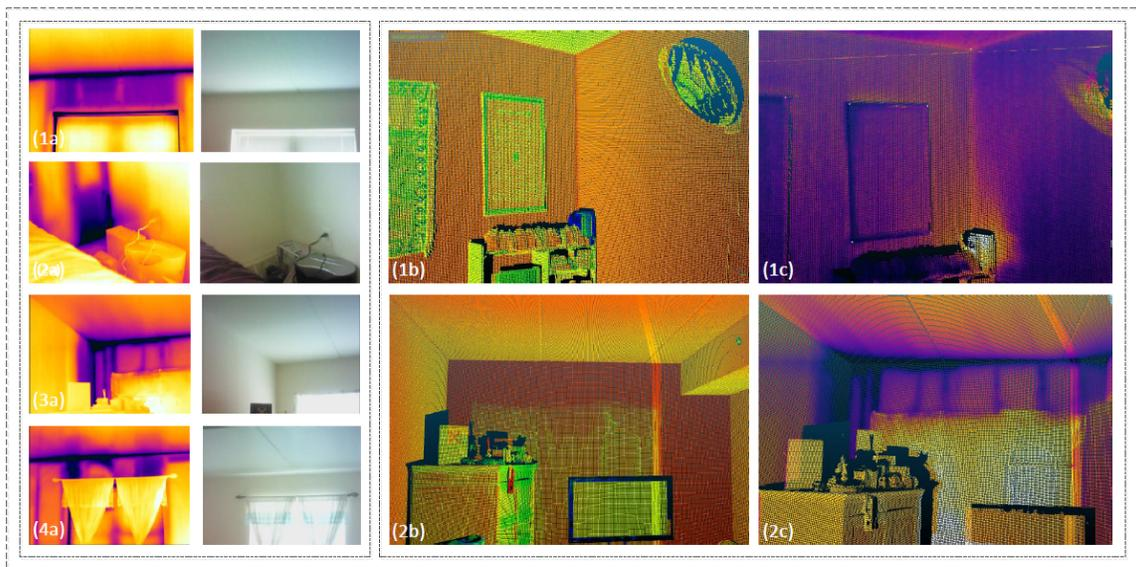
Figure 13. Raw data and 3D thermal point cloud. (a) Infrared thermography and digital images, (b) LiDAR point cloud, (c) 3D thermal point cloud.
