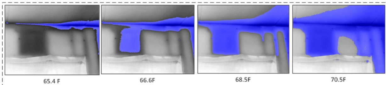
Figure 10. Infrared images with cold alarm (blue area means temperature lower than the threshold value).
