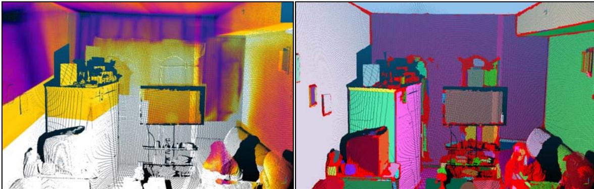
Figure 15. 3D thermal model and segmented 3D point cloud.
