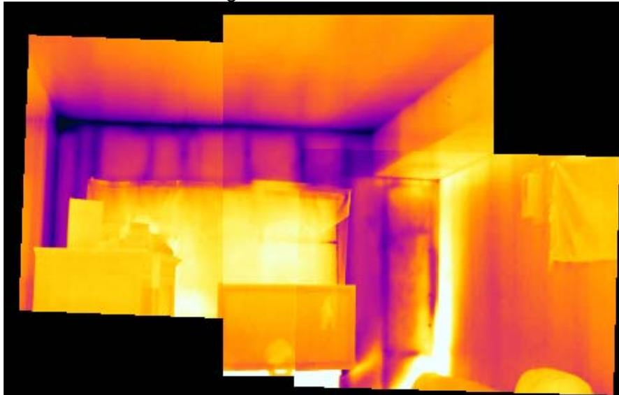
Figure 8. Automatic indoor infrared image stitching result.
