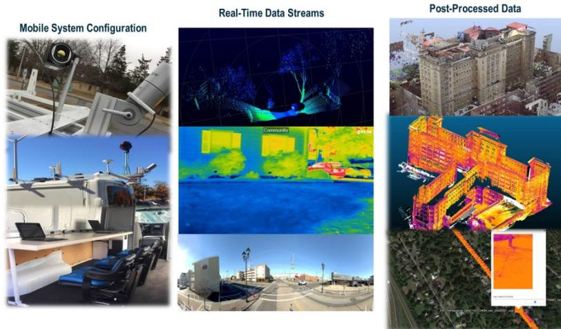
Figure 35. A mobile spatially resolved infrared thermography system.
