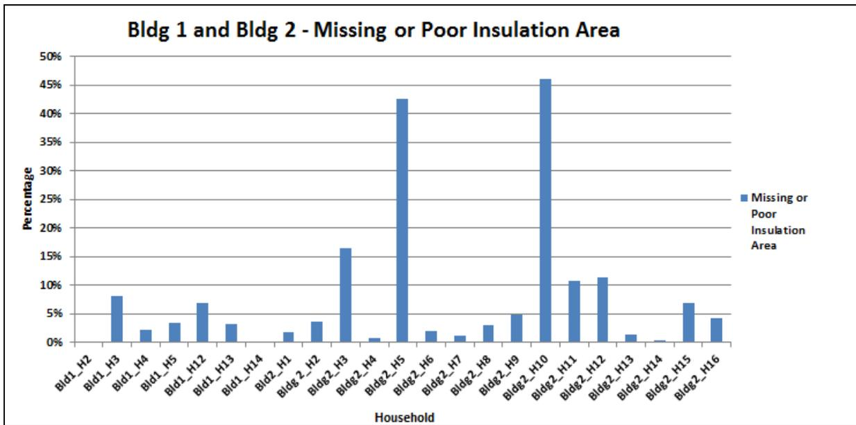
Figure 28. Percent of Poorly Insulated Areas in Apartments in Building 1 and 2.
