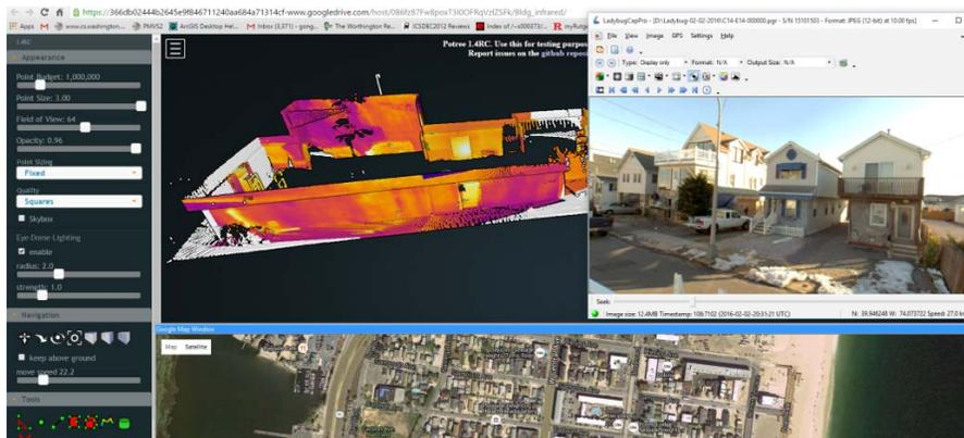
Figure 36 .Web-based visualization of spatially resolved infrared thermography
