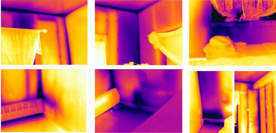
Figure 22. Examples of air infiltration.
