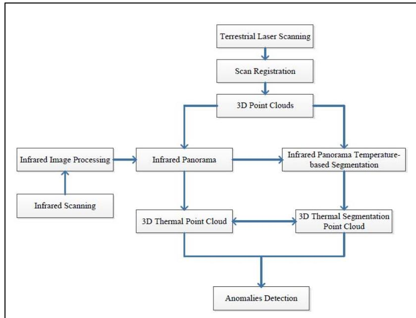
Figure 2. Generation of Spatially Resolved Infrared Thermography and Building Hazard Detection.
