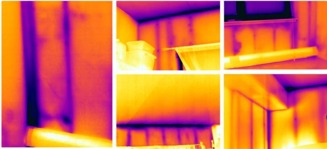
Figure 24 Examples of thermal bridge issues.
