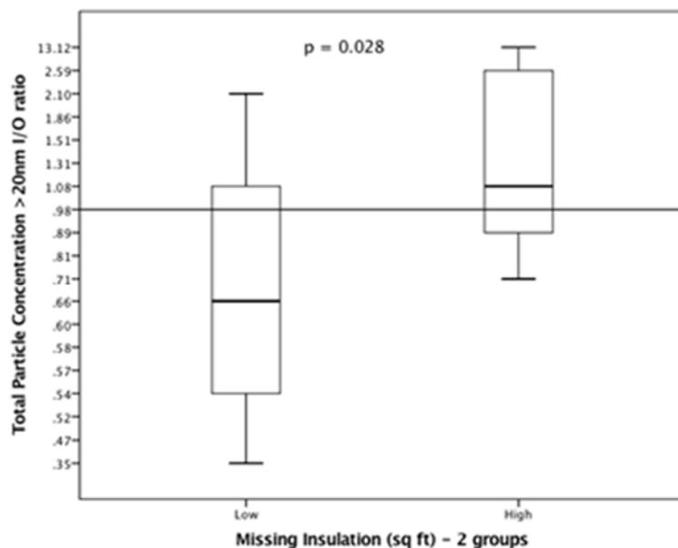
Figure 30. a. Indoor particle number concentration stratified by missing insulation levels (ft<sup>2</sup>). b. I/O particle number concentration ratio stratified by missing insulation levels (ft<sup>2</sup>).
