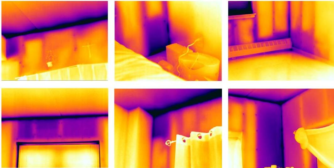
Figure 20. Example Missing Insulation (Sections with missing or poor insulation are indicated by the cooler colors).
