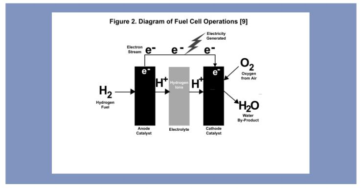
the fuel cell can continue to provide energy so long as a fuel is present. A battery, in contrast, has a finite storage of energy before it needs to be recharged. A graphical depiction of the electrochemical process of turning hydrogen fuel into energy using a fuel cell is shown in Figure 2. All fuel cells contain an anode, cathode and electrolyte. The hydrogen fuel is broken into electrons
