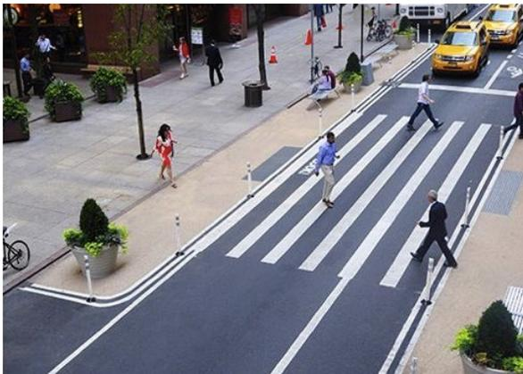
In this example, the pinch-point curb extension was installed at a relatively low-cost by using just paint and plastic bollards.
