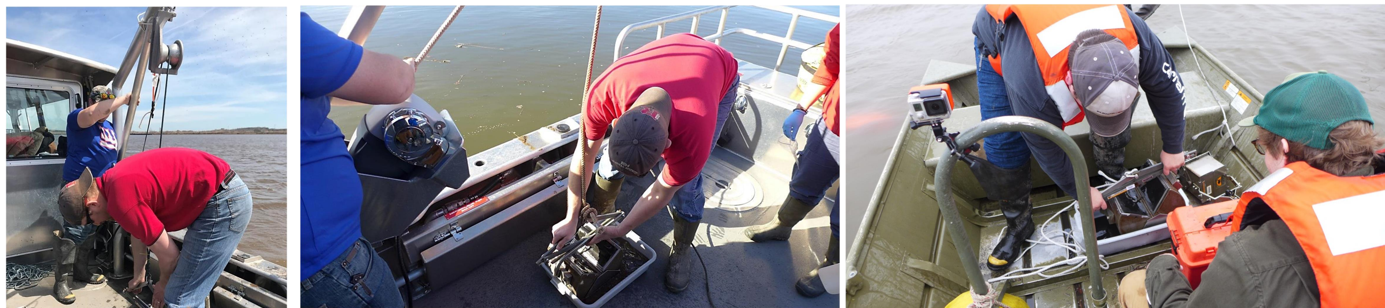
Members of the MERI research team using the Ponar grab sampler on the R/V Rutgers and the Go-Devil shallow water craft. Each sample is a composite of three Ponar grabs.
